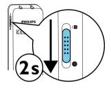
To power off, pull down the power switch on the side of the device 2 again and hold for about two seconds.
